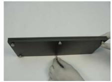
6. Remove mold from refrigerator. Unscrew all six screws to separate the two plates.
