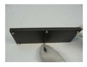
**4.** Screw in all six screws from the <u>bottom</u> of the mold and hand tighten. Mold is ready for use.
