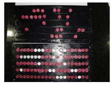
8. Place Top Plate beside the Bottom Plate. Remove any lozenges from the Bottom Plate using a rubber or silicone spatula. Do not use metal tools.
