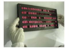
7. Lift the Top Plate to remove lozenges from the mold.
