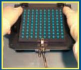
8. To separate capsules, press thumbs down on Filler handles while lifting capsule tray up with fingers. After separation, release cam lever to drop capsule bodies flush with Filler.
