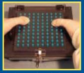
12. Place capsule tray back onto Filler. To lock capsules, push down on locking plate with thumbs while pulling up on lifting plate (not visible) with fingers.
