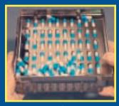
1. Pour 50+ capsules onto Orienter and shake back and forth moving capsules into slots.
