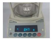
7. Weigh filled Tap DensiMeter. Your tapped density is the final weight. Example 0.47g means a tapped density of 0.47g/ml.
