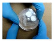
5. Rotate the top disc 90° clockwise to close cavity in middle disk.
