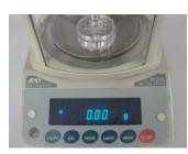
1. Place empty Tap DensiMeter on balance and tare the balance.
