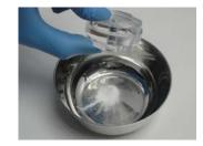
6. Turn over Tap DensiMeter and tap out any remaining powder in the top disc.
