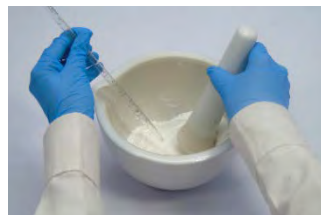
2. Wet powder with a wetting solution suitable for the formulation. Add slowly until the product has a dough-like consistency.
