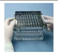
**2.** Replace with the changeover top sheet, aligning the locating post on the base with the locating hole on the top sheet. Finally, reattach parts using hand screws.
