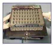
**4.** Push the sliding portion of the Orienter to the left to drop capsules into the Filler.
