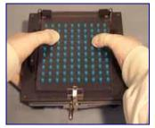
**12.** Place capsule tray back onto Filler. To lock capsules, push down on locking plate with thumbs while pulling up on lifting plate (not visible) with fingers.
