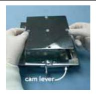
**5.** Lift out the spacer plate and replace with the changeover spacer plate. Be sure the cam lever is pointed at 3 o'clock.
