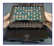
**3.** Open Filler locking plate and place the Orienter locating feet in the holes on the Filler marked "I".
