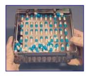
**1.** Pour 50+ capsules onto Orienter and shake back and forth moving capsules into slots.
