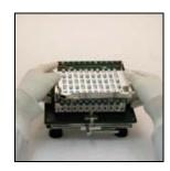
**3.** Open Filler Locking Plate fully by sliding clamp forward. Place Orienter locating feet in the holes on the Filler marked "I".
