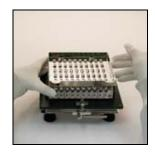
**4.** Push the sliding portion of the Orienter to the left to drop capsules into the Filler.
