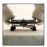
**8.** To separate capsules, press palms down on Filler handles while lifting Caps Tray up with fingers. Remove Caps Tray from Filler. Release Cam Lever to drop capsule bodies flush with Filler.
