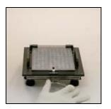
**7.** Close the Filler Locking Plate and slide Locking Clamp to secure. Gently squeeze the Cam Lever toward the post to secure bodies in the Filler.
