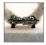
**12.** Place Caps Tray back onto Filler. To lock capsules, push down on Locking Plate with thumbs while pulling up on Lifting Plate with fingers.
