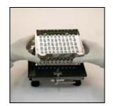
**6.** To fill remaining rows, repeat steps 1-4 except in Step 3 align the Orienter locating feet in the holes marked "II".
