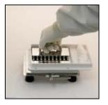
**11.** Use Tamper to pack powder. Spread the remaining powder from reservoir into bodies. All the bodies are now filled. Remove Powder Tray.
